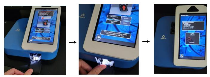
4. When the alignment completes (and prompted to "Enter the Sample" at the top left black bar), open the door to the first stop ( $45^{\circ}$  angle) and pipette  $60\mu$ L of the check bead sample into the loading well in one fluid motion.
