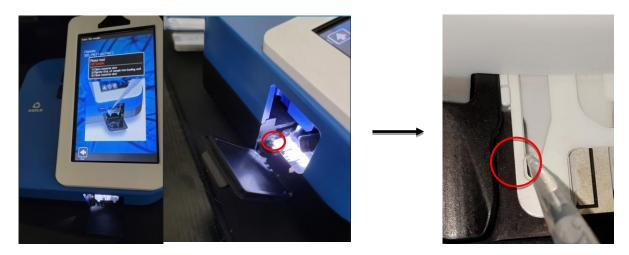
5. Immediately close the door (try not to delay longer than a second or two or the beads will begin to settle). Once the door is closed, the test will automatically run.
