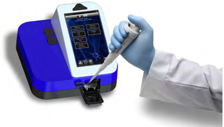
Figure 1 – Orflo's Moxi GO II – Next Generation Flow Cytometer. Image shows user loading a sample into the two-test disposable flow cell. The Moxi GO II is a configurable flow cytometer with a 488nm laser and up to two fluorescence recording channels (2 PMT's with emission filters at 525/45nm filter and 561nm/LP, respectively).
