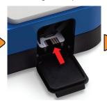
5) Pipette 60uL of Stained Sample Into the Cassett e. Close Door. Test Begins.
